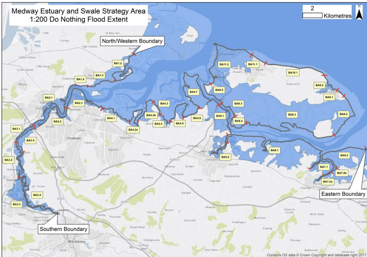
Figure 1: Medway Estuary and Swale Strategy area. The blue line delineates the extent of potential flooding under a 0.5% Annual Exceedance Probability (1 in 200 year) event if no defences were in place. Based on this worst-case scenario approximately 17,226 properties are thought to be at risk of flooding over the next 100 years.
